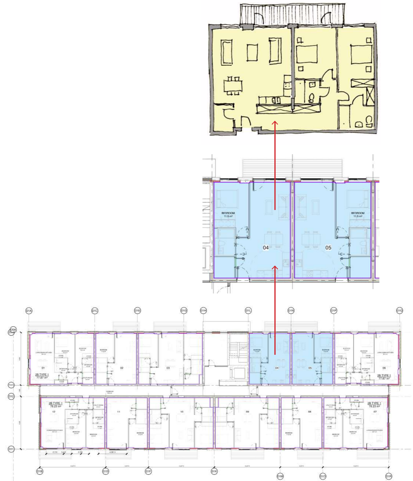
Figure 86 - Example of 2 one bed apartments converted into one 2 bed apartment (Block D1)
