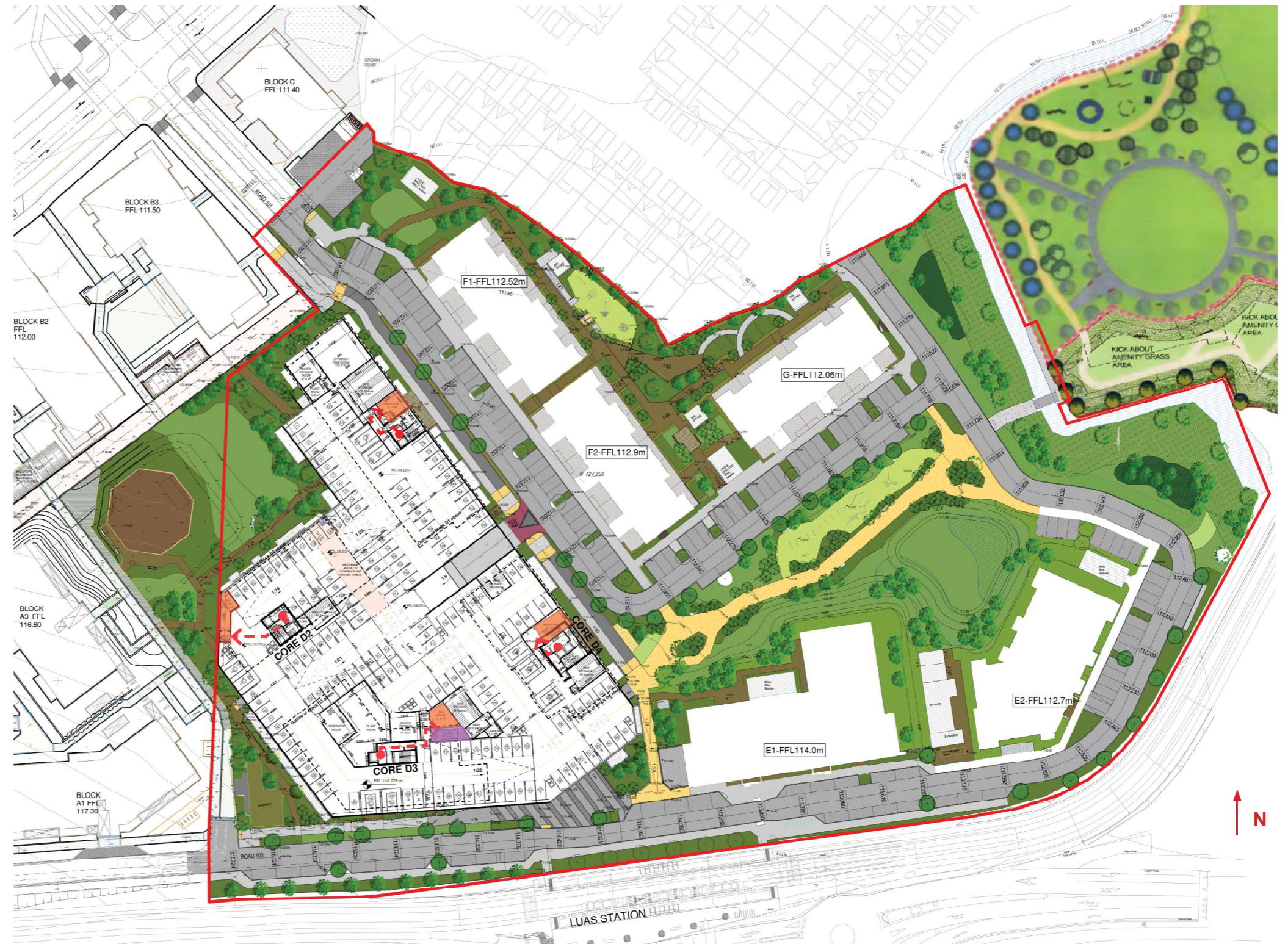
Figure 92 - Basement Floor Plan with waste storage areas noted
